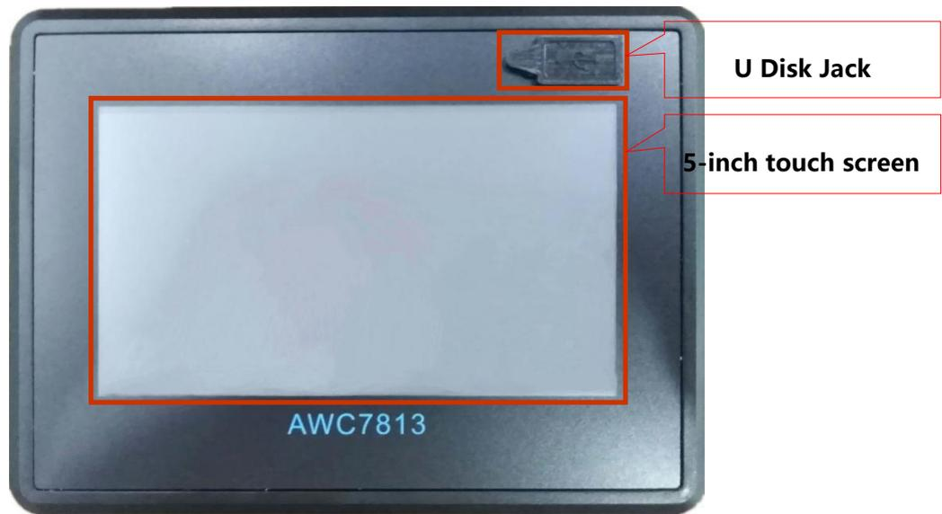
Figure1-5-2 Panel size diagram
