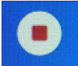
This icon will only be displayed when the machine is working. When the machine stops, this icon will automatically switch to 【Box】 icon. In the [Figure3-1-1 Main interface 1](#), click the 【Stop】 button to stop the running machine, back to position point. If you want to continue processing after stopped file, can click 【Continue to Previous Work】 . For details, please refer to [3.25.3 Continue to Previous Work](#).
