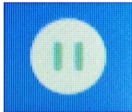
The icon is displayed when the machine is working. In the [Figure3-1-1 Main interface 1](#), click 【Pause】 button, the machine pauses and maintains its current state. After pressing this button, except for the 【Stop】 key, all the other keys cannot be used. Press this key to set the speed and power of the file being processed. For details, please refer to [3.9.2 Modify the speed of the file being processed](#)、[3.10.2 Modify the power of the file being processed](#)。
