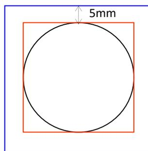
Assuming that the cutting graphic is a circle, the cutting frame graphic is a red rectangle. If the 【Blanks Distance】 is set to 5mm, the cutting frame graphic is a blue rectangle, that is, the distance from the actual cutting frame position is 5mm.
